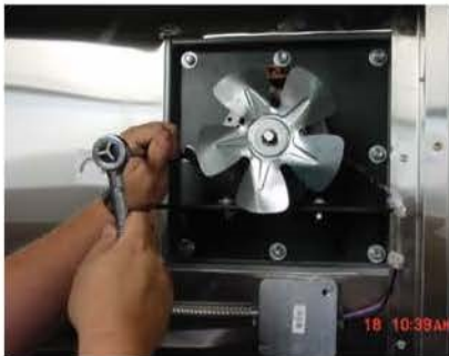
Step 4 - Loosen Nuts from the Convection Fan Motor Mount(s).
