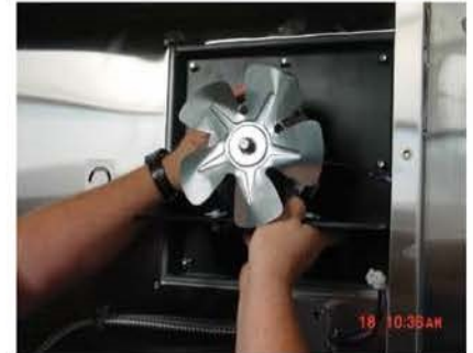
Step 6 - Place a Firm Hold on the Motor Mount & Motor...
