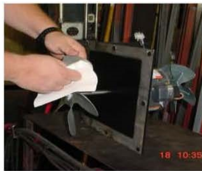
Step 8. - Clean Fan Assembly(s) Completely. Check Set Screws and Inspect Blades for Signs of Imbalance or Irregularities. You are now ready to reassemble.
